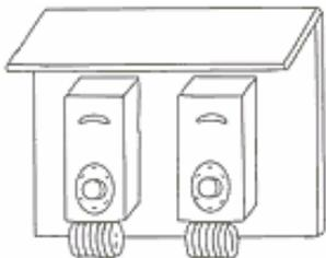
To get the desired temperature, thermostats should be located at plant height near the center of the greenhouse where they are not influenced by drafts or sidewall cooling. It is best if both the thermostat and speed control are located together and protected from direct contact with sunlight and water. One simple way to accomplish this would be to mount the controls to a piece of wood with a top on it like in the picture to the left. Wood should be painted white to shade it from the sun.
