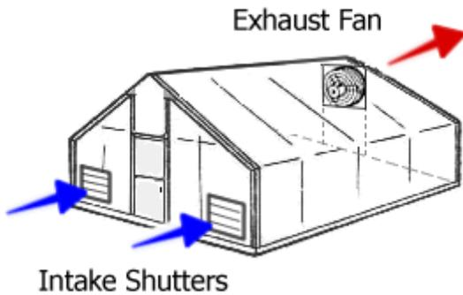
The picture to the left shows optimal fan and shutter placement in a greenhouse. The exhaust fan should be mounted near the peak so that it is exhausting the hottest air in the greenhouse. The intake shutters should be mounted on the opposite end of the greenhouse so that the cooler fresh air travels across the entire structure minimizing hot spots.
