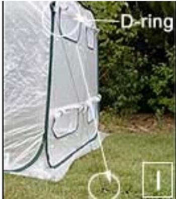
**Step 8:** Secure your DreamHouse™ using the high-wind tie-downs. Insert one end of the rope through the D-ring in the top corner, then through the anchor. Knot the rope around a stake and insert it in the ground at a 45° angle. Keep as much tension on the rope as possible. Repeat this step with all corner locations, as well as the D-rings on the peak ends and top center of the side walls.
