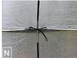
**Step 11:** Repeat Step 10 with the second L-shaped fiberpole. When the poles are completely assembled, move them to the center of the wall, and tie them to hold them in one place. See photo "N").
